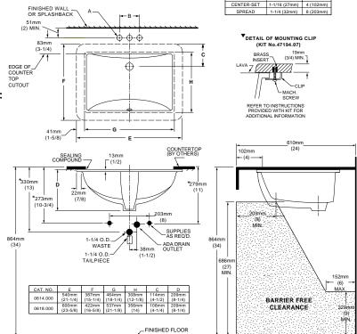
Countertop 864mm (34") from finished floor. Lavatory installed 102mm (4") from front edge of countertop. Countertop thickness to be 25mm (1") maximum.
